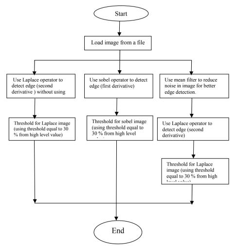
Figure.6 Block diagram of designed algorithm.
