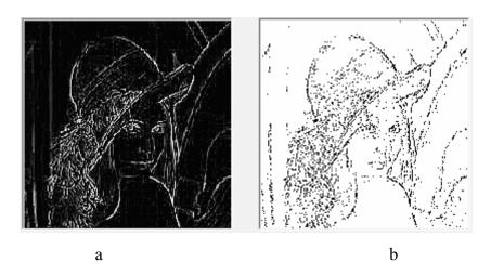
a Figure.8 a. Result of Laplace Operator . b. Laplace Image Threshold.
