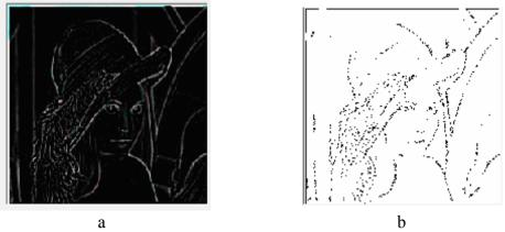
Figure.11 a. Result of Laplace Operator after using Mean Filter. b. Laplace Image Threshold.
