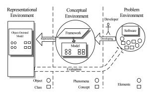
Fig 4. General Object Oriented Software Model.
